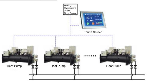
Standard MODBUS interface, compatible with various engineering building control systems.
