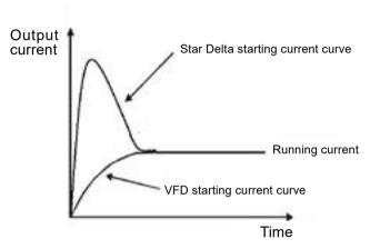
Comparison starting current curve between VFD and Star Delta
