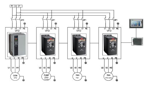
VFD Compressor + VFD Water Pump + VFD fan + VFD AHU
