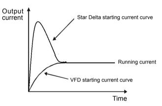
Comparison starting current curve between VFD and Star Delta
